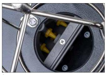
. Removing the filter and coalescing filter provides access to the Second Stage Venturi Shut off Valve through the hole in the cover. Inspect and ensure it moves freely. If it does not move freely, or if the shut off valve is damaged, ripped or torn, follow the next steps for replacing.
