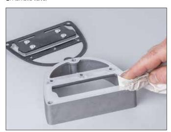
. Clean the gasket surfaces on the base and vacuum generating engine.
