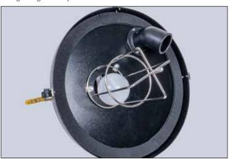
**5**. On 30 & 20-gallon vacuums, be sure to line up the scallop in the gasket with the vacuum exit elbow.
