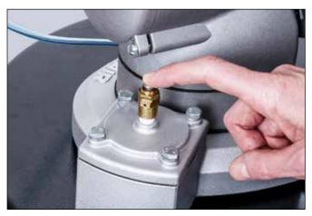
**2**. Actuate the pulse by momentarily pressing the push button valve. Actuate the pulse 3 to 10 times, waiting 2 seconds between pulses.
