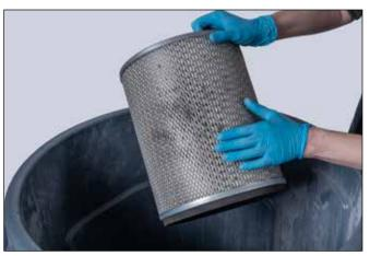
**5**. Clean the filter by shaking and tapping the filter, or by directing compressed air against the interior surface of the filter.
