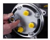
4. Install new nozzles using a 5/8" socket. Finger tight will suffice.
