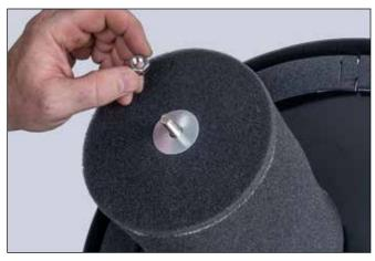
. Remove nut and washers holding the wire cage coalescing filter in place.
