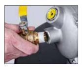
1. Install the ball valve onto the PowerQUAD Vacuum Generating Engine. Use Teflon tape or thread sealant on the threads of the ball valve.
