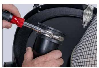
**3**. To replace, remove the reverse flow check valve by removing the worm-gear clamp.
