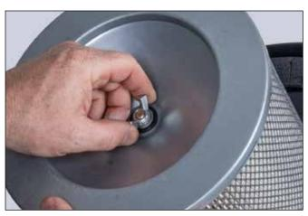
. Remove the wingnut and sealing washers at the bottom of the filter.
