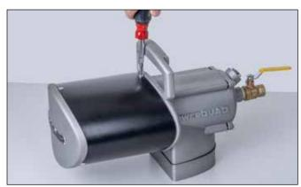
1. Remove the three (3) screws securing the exhaust housing.
