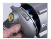
2. Remove the manifold. Gently rotating the manifold left and right while puling the manifold out of the body may be needed.
