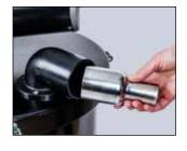
2. Install the vacuum hose adapter into the inlet elbow. If needed use a rubber mallet to tap the adapter into the inlet elbow.
