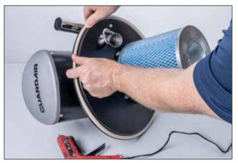
**4.** Work around the vacuum cover dispensing fresh hot glue while pressing the gasket down into the fresh hot glue.
