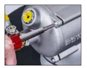
1. Remove the four manifold screws.
